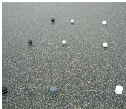
Figure 7: FOD targets of different shades used to evaluate visual detection systems
