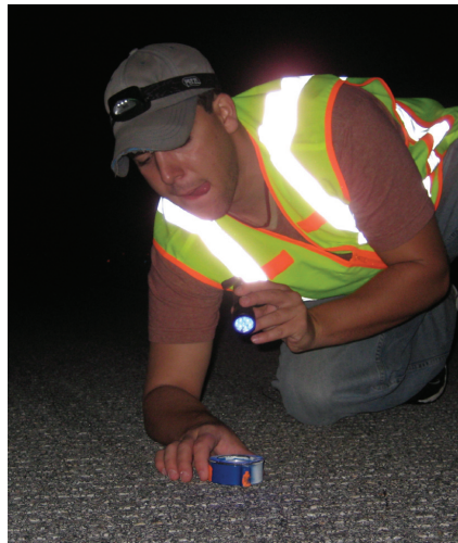
Figure 3: CEAT researcher positions a piece of FOD for nighttime testing
