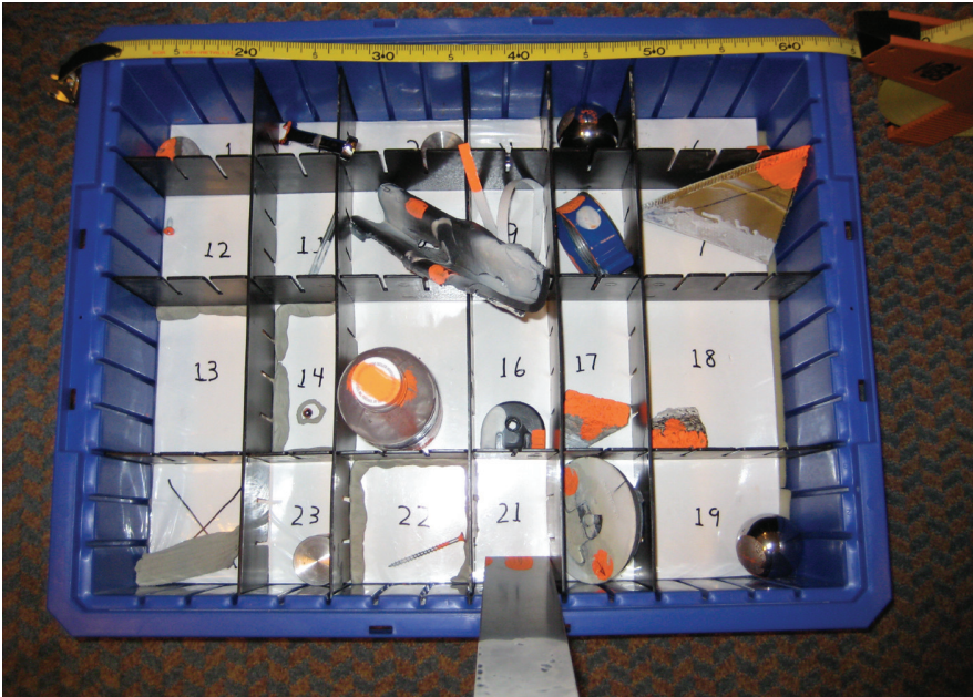
Figure 2: Collection of FOD items used by researchers in evaluation of detection capabilities
