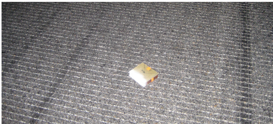
Figure 4: An example of larger piece of FOD being used for blind detection evaluation
