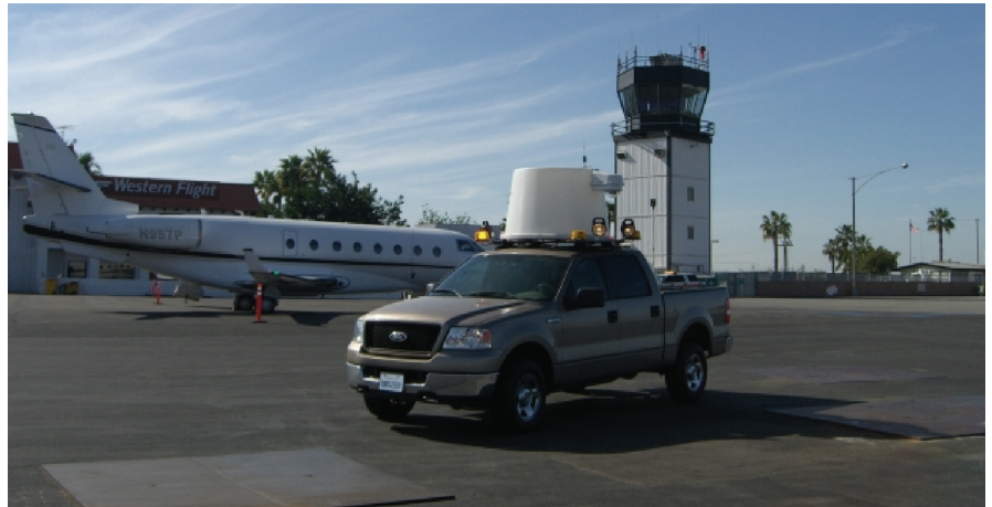
Figure 6: Mobile FOD Detection Technology developed by Trex Enterprises
