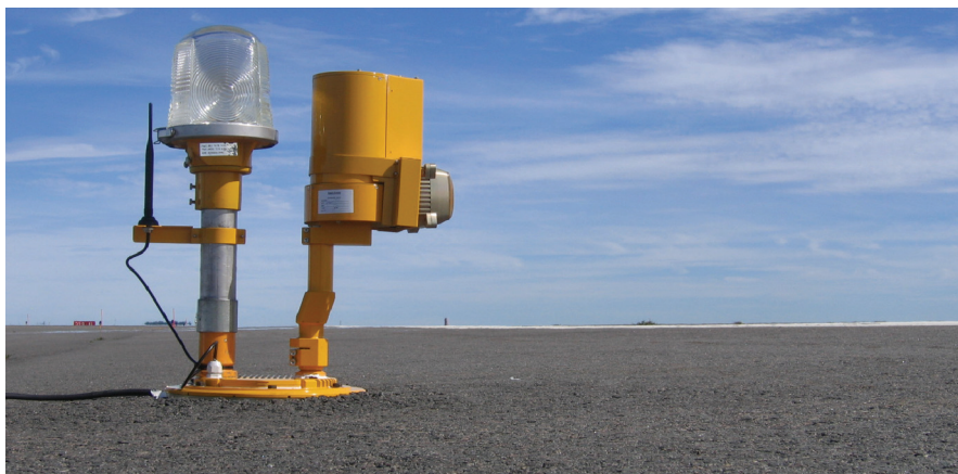
Figure 5: XSight’s FODetect Surface Detection Unit in place on the edge of a runway
